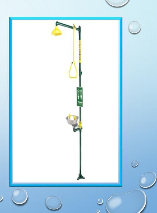
COMBINATION SHOWER WITH SE-690 EYE/FACE WASH WITH DUAL SPRAY OUTLETS, FLIP TOP DUST COVERS AND STAINLESS STEEL BOWL. PAINTED GALVANIZED STEEL STANCHION WITH AN IMPELLER ACTION DELUGE SHOWERHEAD ACTIVATED BY A HIGH VISIBILITY YELLOW PULL ROD.
