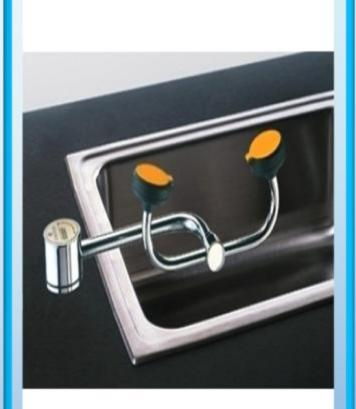
APPLICATION: AUTOFLOW EYE/FACE WASH FOR MOUNTING ON COUNTER NEXT TO SINK. SWINGING THE SPRAY HEAD ASSEMBLY 90 DEGREES HORIZONTALLY OUT OVER SINK ACTIVATES THE WATER FLOW. THE UNIT REMAINS IN OPERATION UNTIL THE SPRAY HEAD ASSEMBLY IS SWUNG BACK INTO THE STORAGE POSITION, CLOSING THE VALVE.
