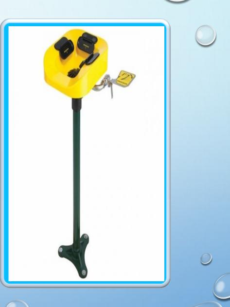
EYE/FACE WASH, PEDESTAL MOUNTED, YELLOW PLASTIC BOWL. TRADITIONAL SERIES ROUND BOWL EYE/FACE WASH STATIONS FEATURE STAY OPEN BALL VALVE WITH PADDLE HANDLE OPERATION AND DUAL SPRAY HEADS WITH AUTOMATIC FLOW CONTROLS AND FLIP TOP DUST COVERS. THE SOFT FLOWING EYE/FACE WASH PROVIDES WIDER COVERAGE, CLEANING FULL FACIAL AREAS. MEETS ANSI Z358.1
