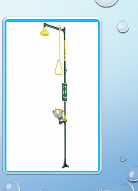
COMBINATION SHOWER WITH SE-693 EYEWASH WITH DUAL AERATED SPRAY OUTLETS, FLIP TOP DUST COVERS AND STAINLESS STEEL BOWL. PAINTED GALVANIZED STEEL STANCHION WITH AN IMPELLER ACTION DELUGE SHOWERHEAD ACTIVATED BY A HIGH VISIBILITY YELLOW PULL ROD.
