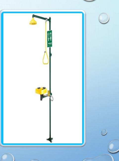
COMBINATION STATION WITH SE-695 EYE/FACE WASH WITH DUAL SPRAY OUTLETS, FLIP TOP DUST COVERS AND YELLOW PLASTIC BOWL. PAINTED GALVANIZED STEEL STANCHION WITH A DELUGE SHOWERHEAD. ACTIVATED BY A HIGH VISIBILITY YELLOW PULL ROD.
